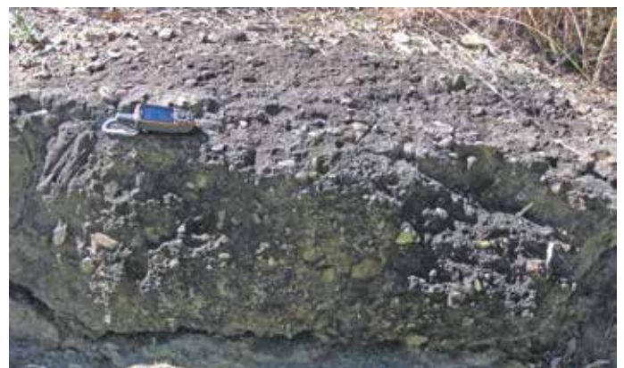
Pt. 8. Pebbly sandstone in the east wall of a cutting, typical of the Esk Formation.
