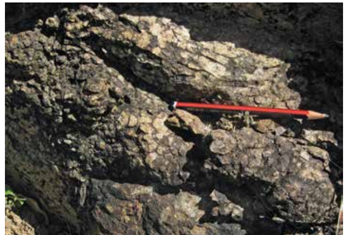
Pt. 7. Brisbane Valley Porphyrite with 1-3 mm crystals in a finer groundmass. The rock also exhibits breccia texture.
